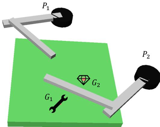
**Fig. 1:** Pick-and-Place scenario studied in this work. Here, two independently controlled agents  $P_1$  and  $P_2$  are each assigned the task of reaching an object,  $G_1$  and  $G_2$  respectively, and then to move back to the initial position. The agents aim to complete it without collisions. Actions of one agent can severely limit the possible actions for the other in this small shared workspace.
